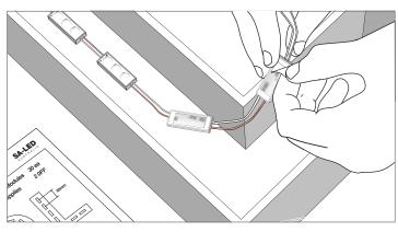
Remove the tape from the back of the LEDs and stick them in place according to the provided layout, including the appropriate module pitch (refer to Figure 1 on page 2).
