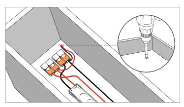
**5** Drill holes along the edge of the channel letter or lightbox connect to the power supply. Wire both ends of LED modules to the power supply (refer to page 2).
