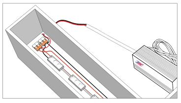
**6** For multiple series, connect them in parallel to avoid voltage drop and ensure even brightness.
